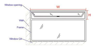
NOTE:- the 'Spa 20' and 'Spa 200' Screen rail is 40 mm. Check to make sure it does not interfere with anything (ie - window handles)
